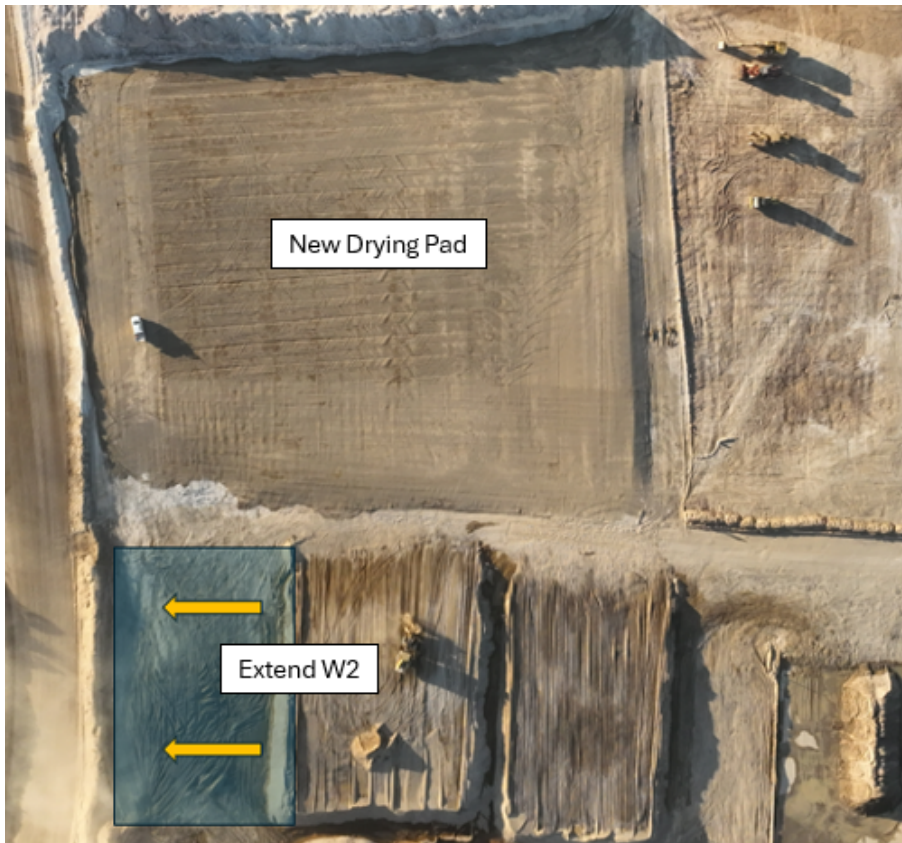
Image 2: Northern drying pads. Used for <12% moisture for final solar drying. Status: 19 th May, Complete
