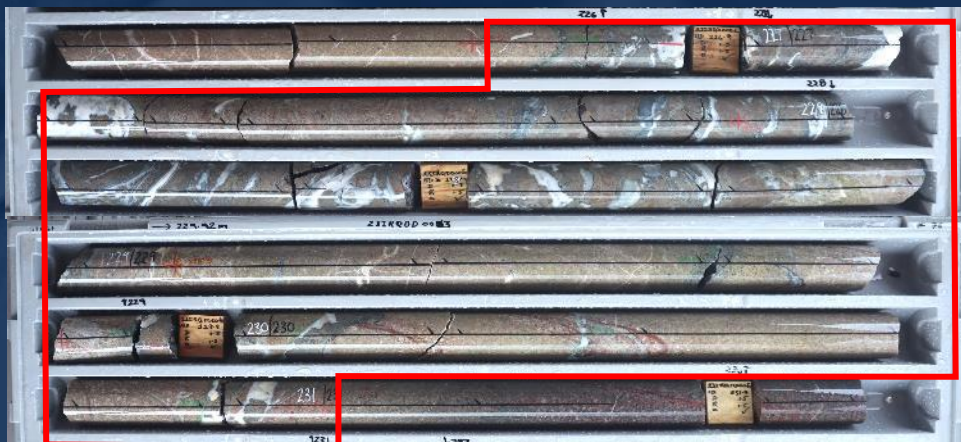
4.3m @ 27.3% Zn, 0.1% Pb and 19.9g/t Ag from 226.7m (IQDD003)
