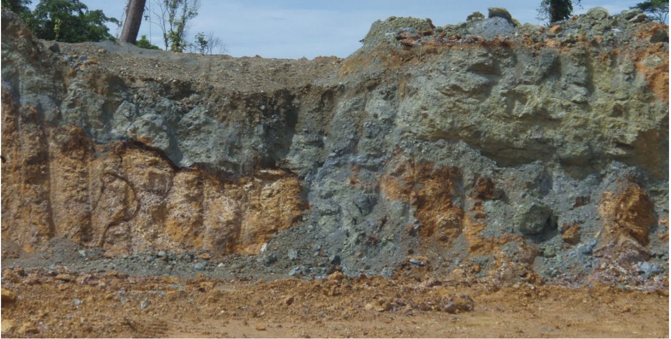
Figure 1. Example of the highly variable degree of oxidation at Simberi which results in material that can be either CIL-treatable (oxide-like) or where less oxidised requiring a different type of processing technology such as flotation to produce a saleable gold concentrate. In this example sulphide material is overlying oxide material.
