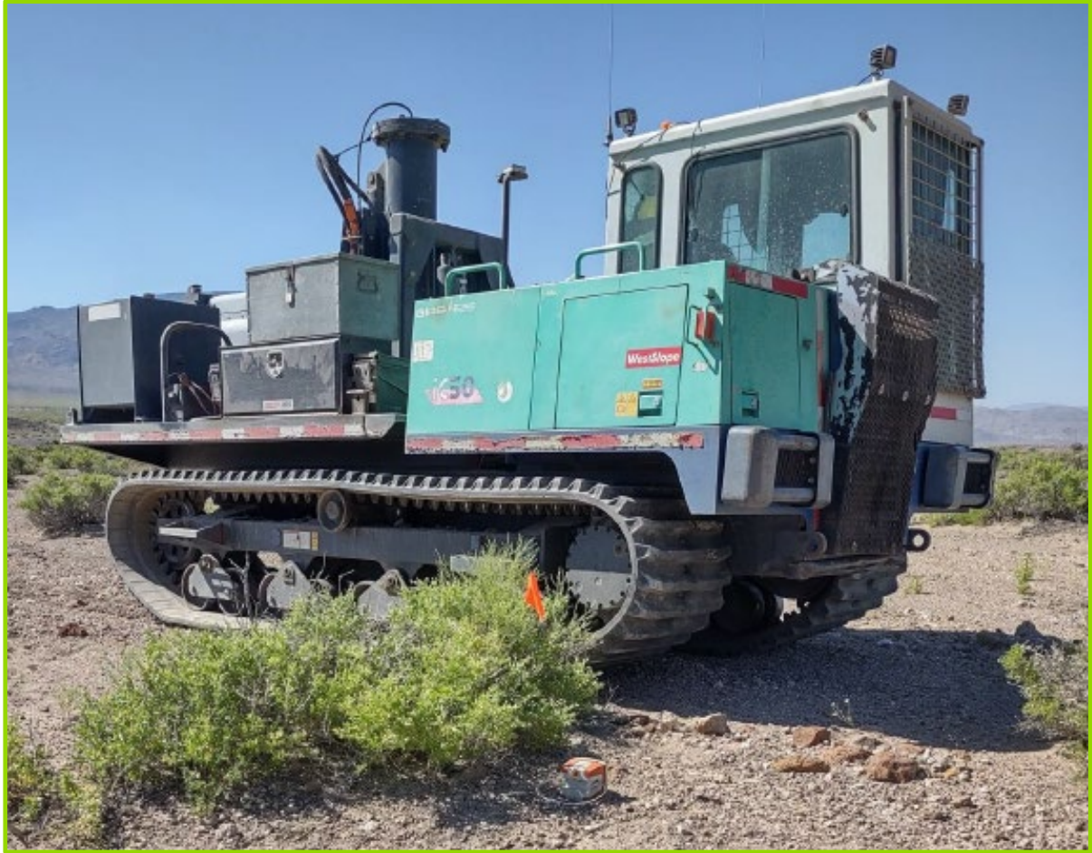
Figure 6: Accelerated weight drop seismic survey source.
