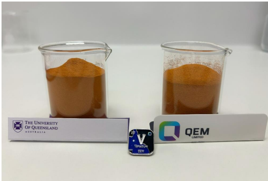
Figure 1 - High purity (99.93%) vanadium pentoxide (V2O5) extracted from Queensland industrial waste at The University of Queensland.
