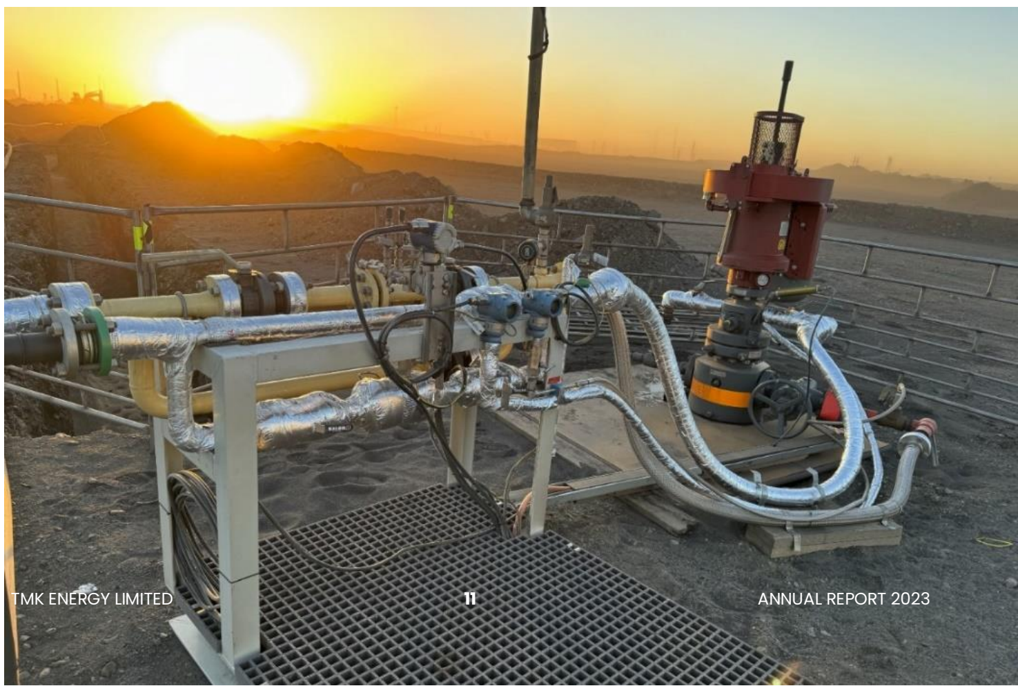
Lucky Fox-1 winterised wellhead and meter skid
