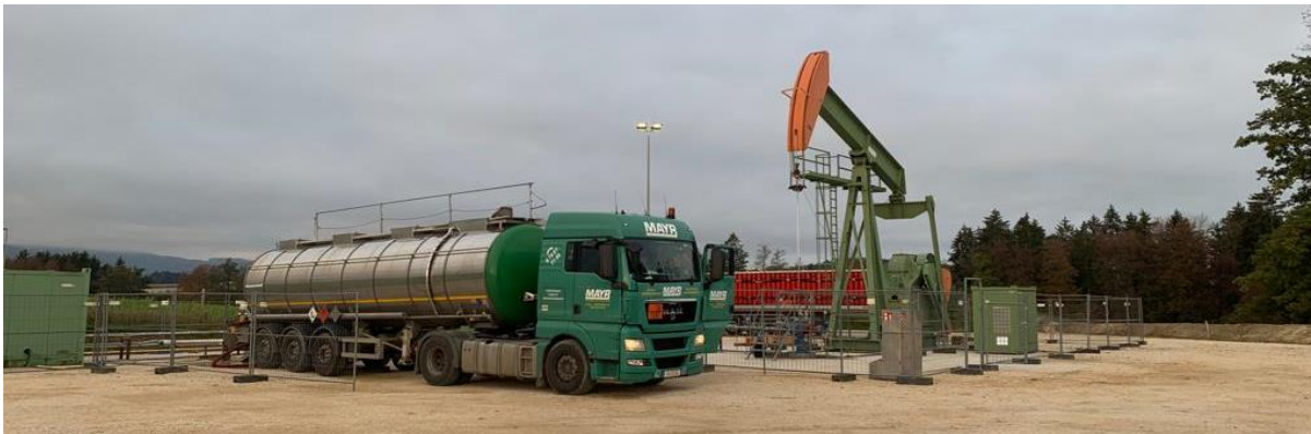
Oil Tanker Loading during Anshof-3 Long term Production Test, ADX-AT-II licence in Upper Austria
