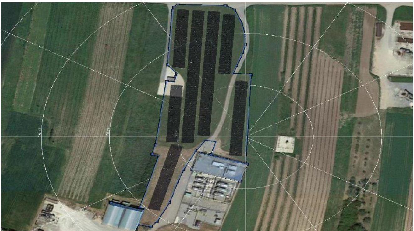
Potential layout of the PV panels at the Gaiselberg site (approx. 1 MWp)
