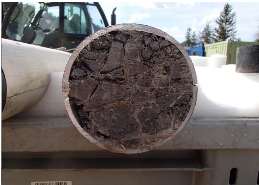
Figure 1: Image of the cut section of recovered core showing the presence of a natural fracture system which is essential for gas production performance
