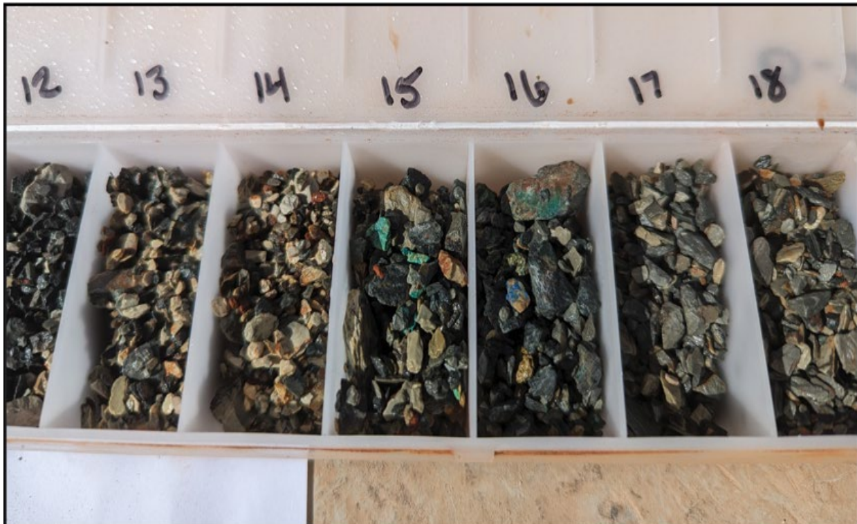
Figure 4 – Chip tray showing BRC004 copper oxide intersection samples (3m @ 6.2% Cu from 13m) with copper oxide minerals malachite and azurite clearly visible.
