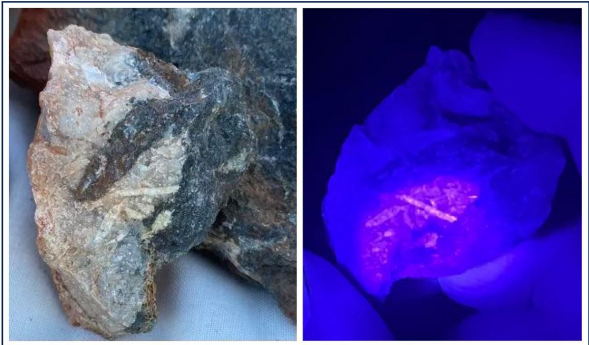
Figure 4. – Hand-specimen of spodumene crystals in LCT pegmatite showing strong pink fluorescence, a characteristic feature under long-wavelength UV light. See location of sample in Figure 5.
