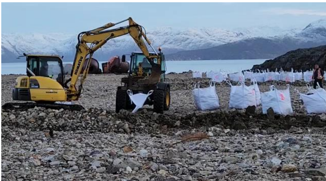
Figure 14: Collecting several tonnes of bulk samples from 5 trenches in the mineralized dumps.
