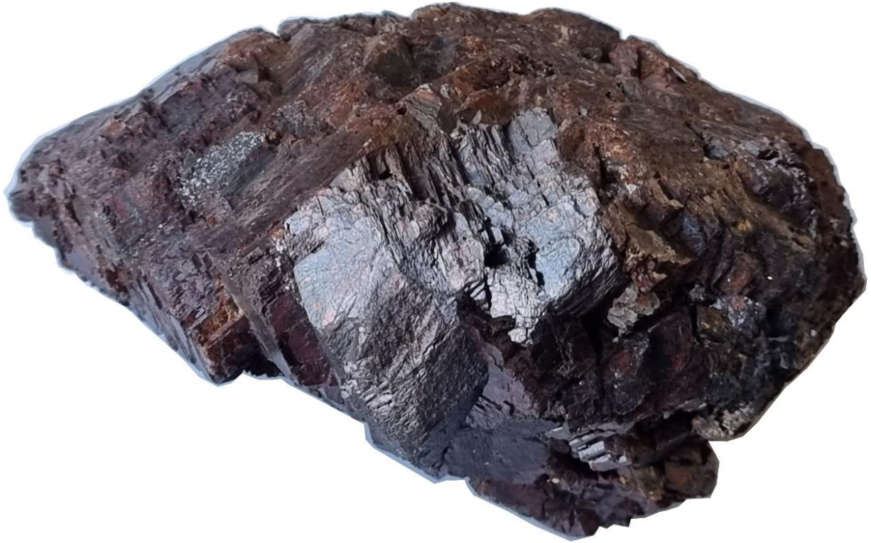
Figure 17: Mineralised waste dump specimen visually estimated to consist of 90% siderite and 10% cryolite.
