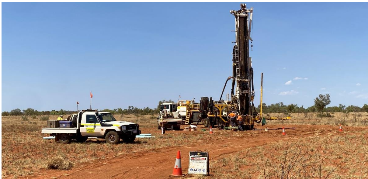
Figure 2. Photo of RC Drill Rig onsite at Quartz Hill.
