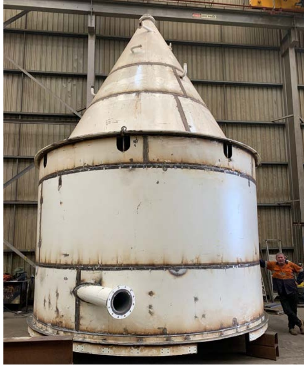
Spray Roaster Oxide Bin workshop fabrication complete
