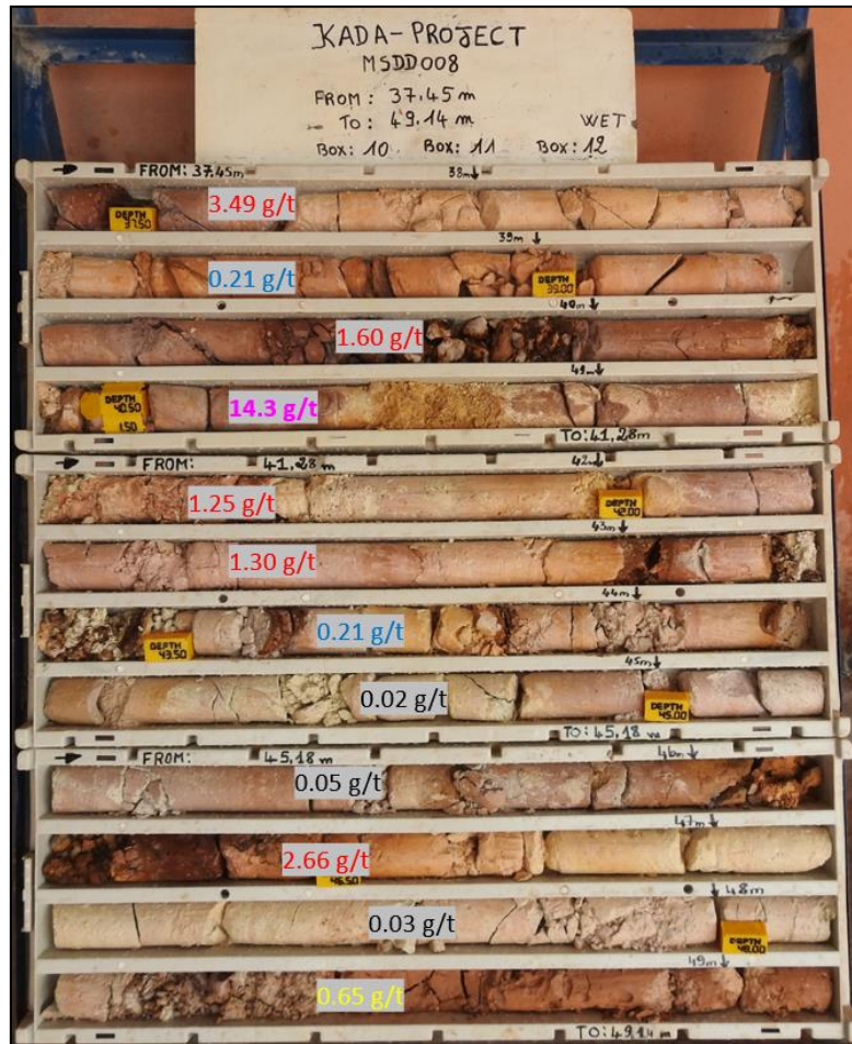
Figure 1: MSDD008 with gold grades across a portion of 29m @ 1.2 g/t intersection from 29m.
