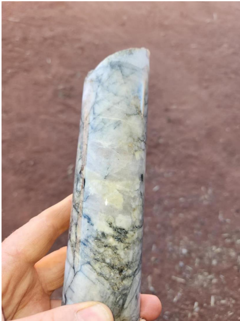
Figure 2: MPDD003 Drill core, from 68.8 m, MPL21-656 (0.02% \text{Li}_2\text{O} ), a Monzogranite made up of roughly 30:30:30 Plagioclase : Quartz : Microcline, the remaining 10% being Muscovite. The yellow/greenish minerals in the sample appear to be saussurite, a potential hydrothermal alteration product.
