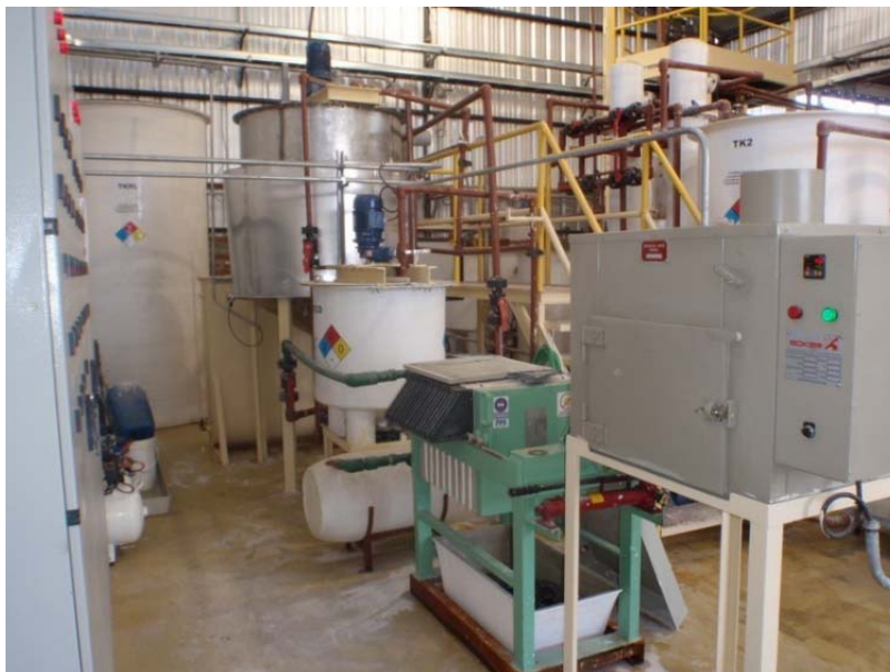
Figure 11: Pilot Plant interior view in original location showing dryer and filter press
