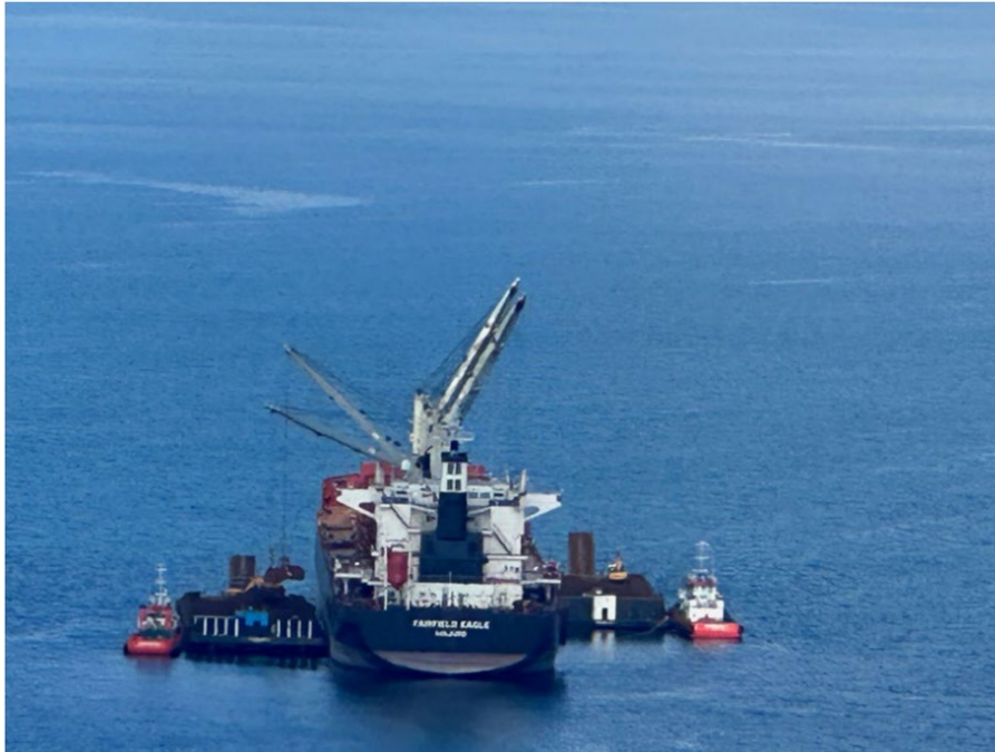
Photo 3 – Loading of Kolosori nickel DSO showing barges on each side of the ship
