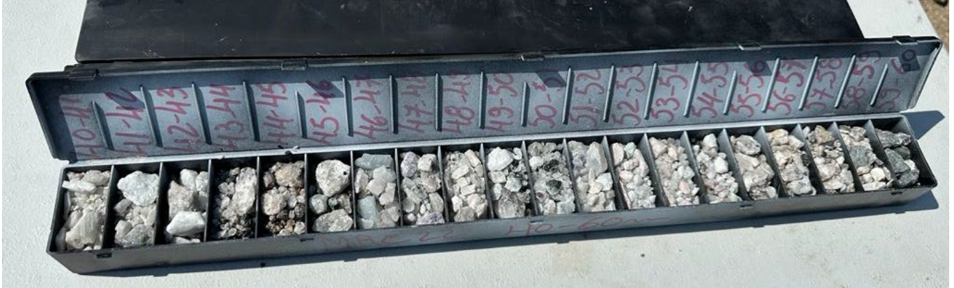
Figure 5: Chip-tray of 40m-60m interval of MRC22. The minerals present include spodumene (10%-20%), lepidolite (1%-5%), elbaite (1%-3%), cleavelandite (variety of albite feldspar, 20%-40%), microcline (variety of potassium feldspar, 5%-10%), muscovite (variety of mica, 5%-10%), and quartz (20%-30%).
