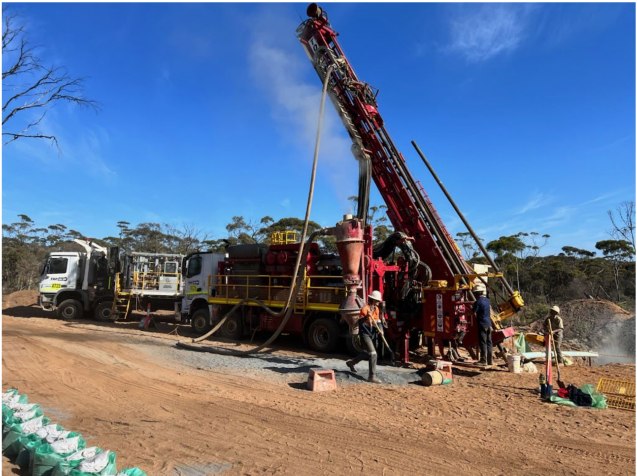
Figure 2 — RC drilling on site at Galileo's 100% owned Norseman project
