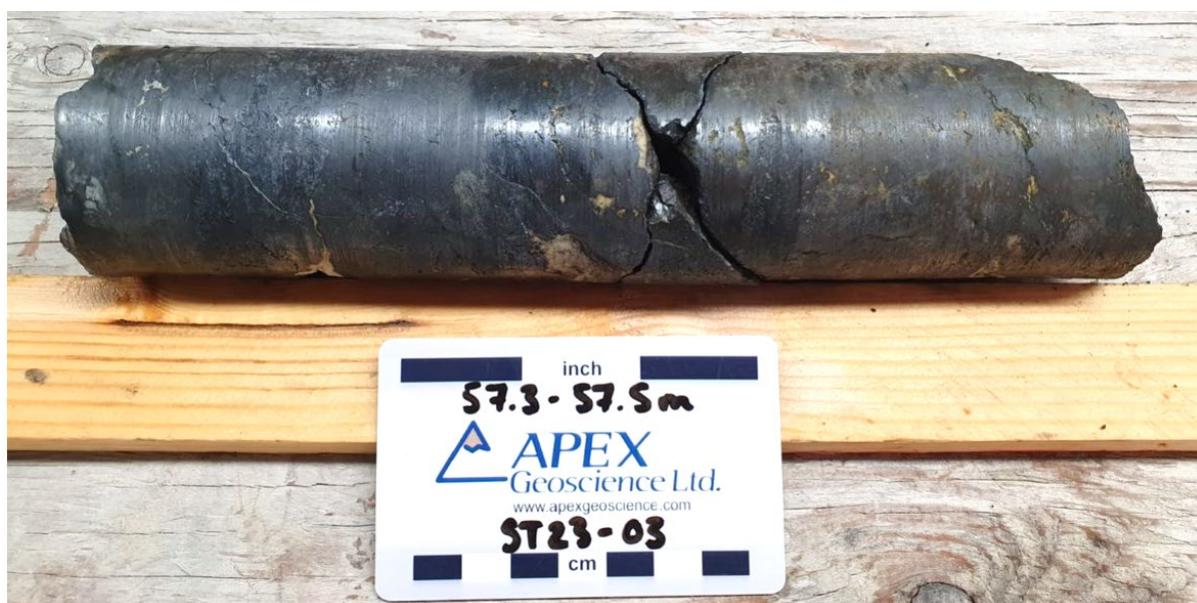
Figure 7: Massive chalcocite (dark grey) in drill hole ST23-03 from approximately 57.4m downhole. This is part of an interval of 57.2 – 57.7m @ 49.6% Cu.
