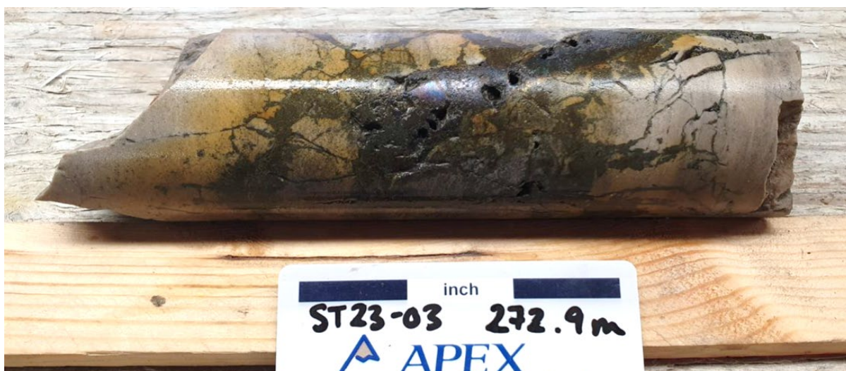
Figure 13: Breccia chalcocite (dark grey), bornite (purple/grey) and chalcopyrite (brassy) in drill hole ST23-03 from approximately 272.9m downhole.
