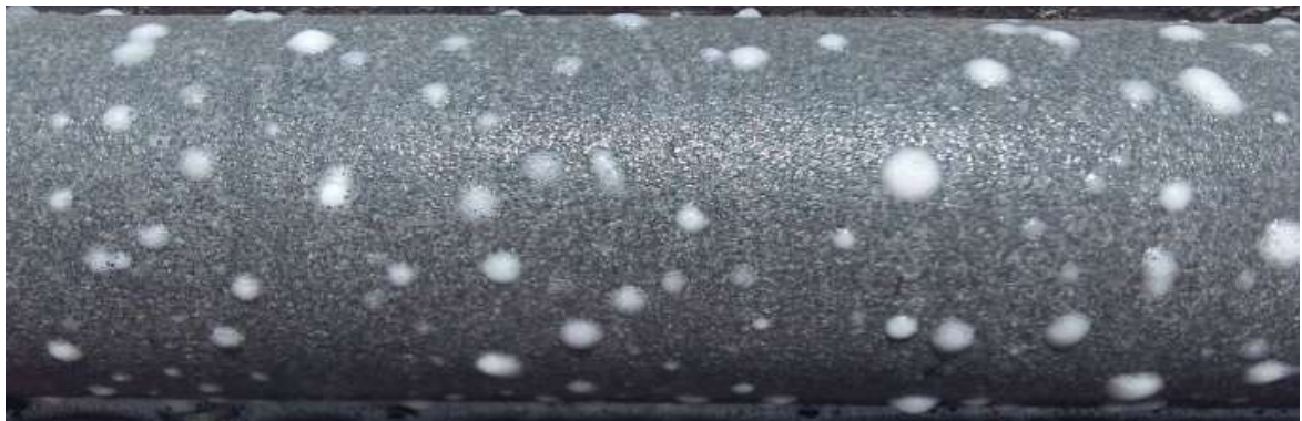
Figure 10 – Gas bubbles on a core sample from ~600m
