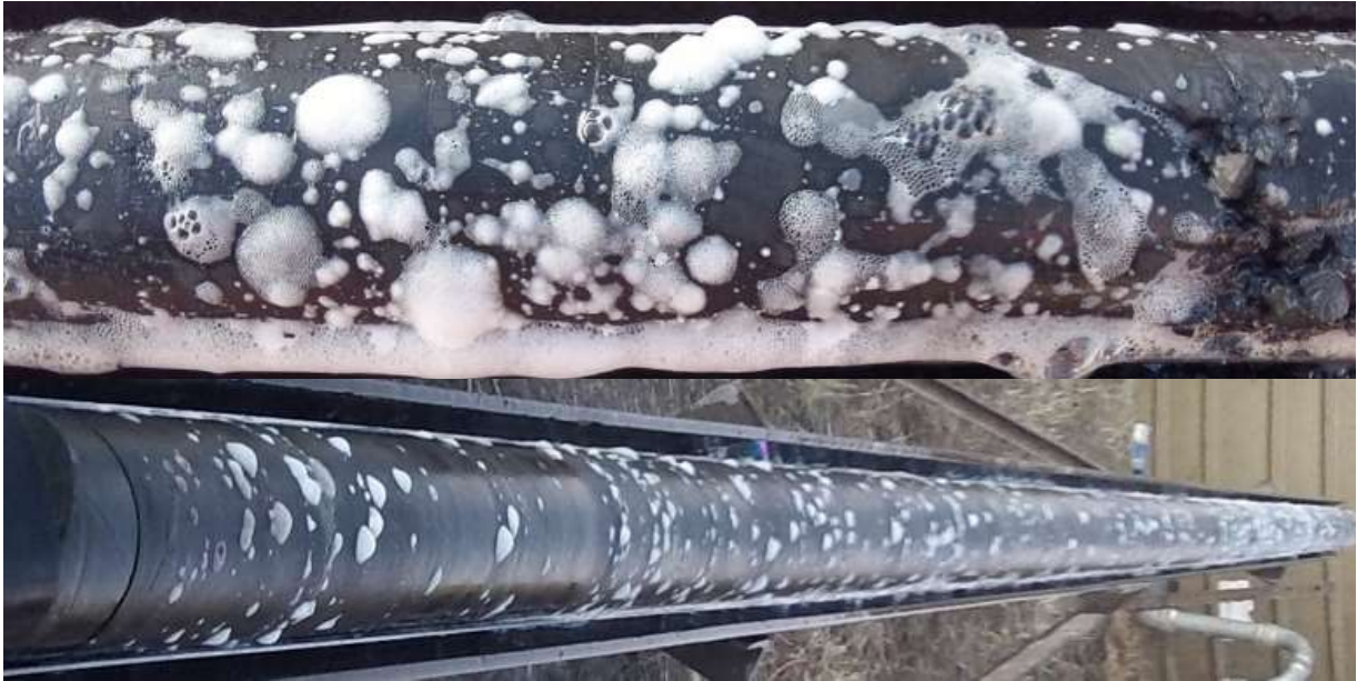
Figure 4 – Core well 270-01C visible gas emissions observed from representative core samples at depths between 155-166m
