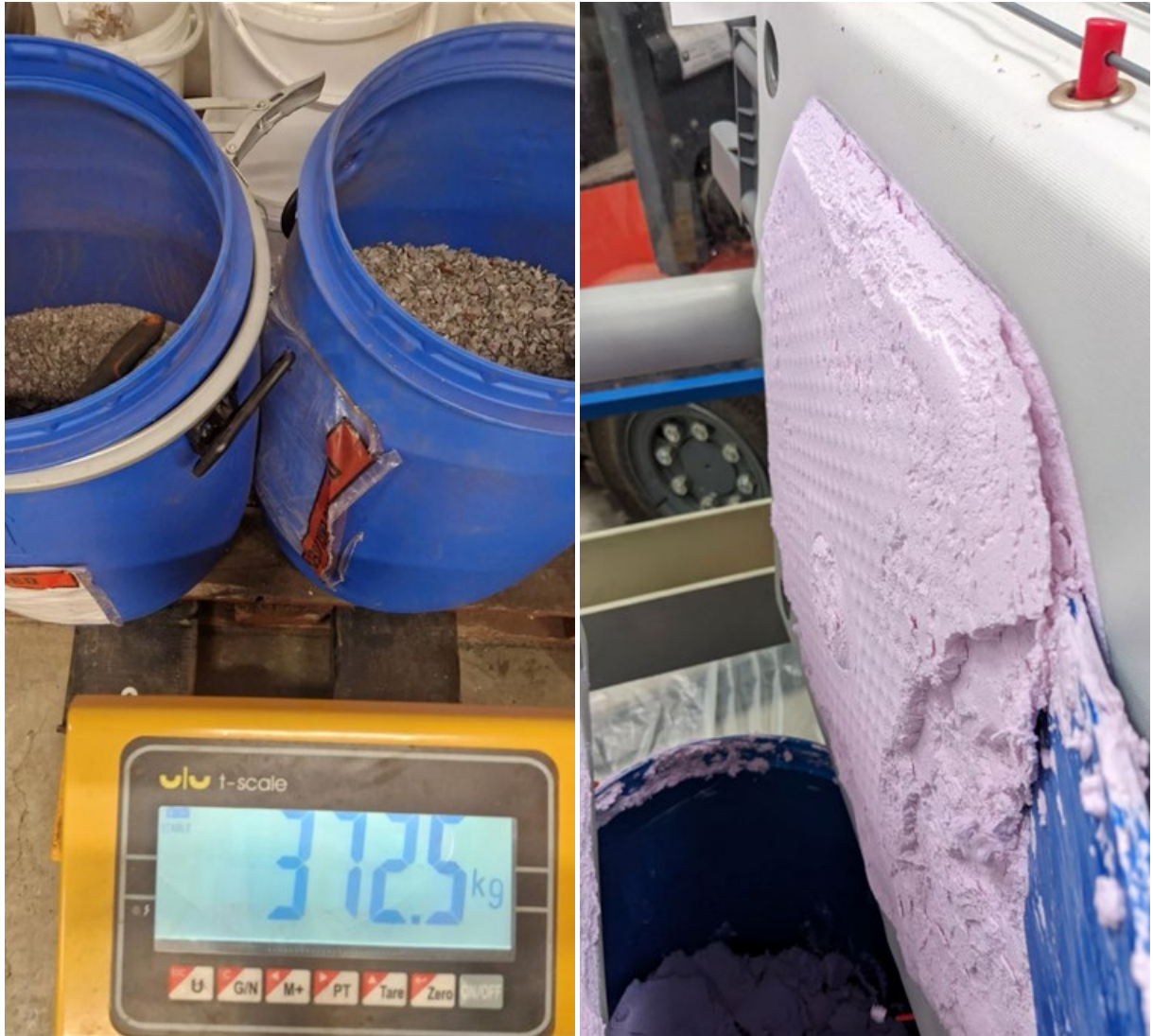
Figure 9: Left, crushed magnets prepared, and right, mixed rare earth filter cake prepared for downstream process commissioning activity.
