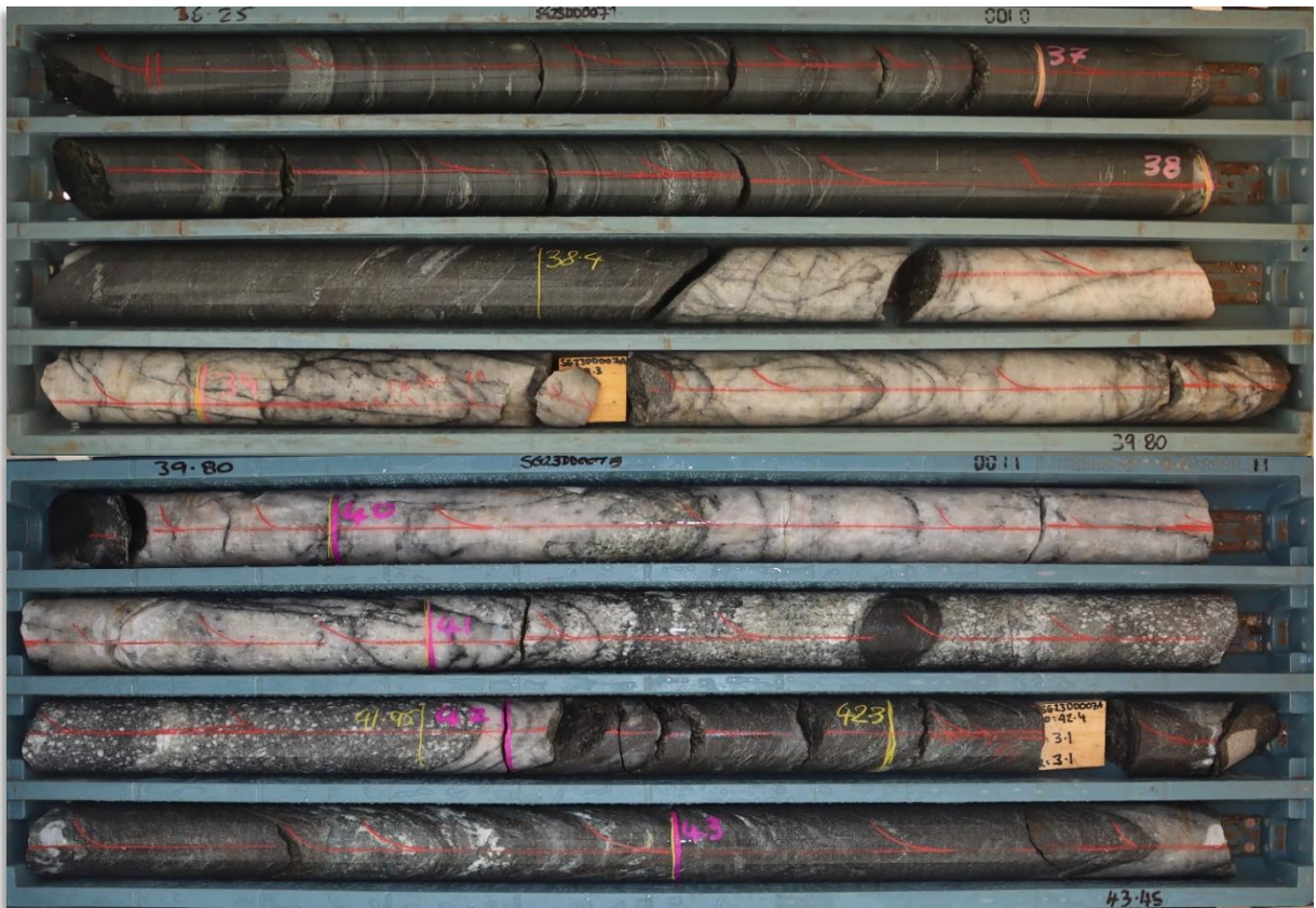
Figure 4: Drill core from SG23DD007 from 36.25m to 43.45m showing Norseman-style quartz lode mineralisation with disseminated sulphide between 38.4m to 41m @ 9.85g/t Au.
