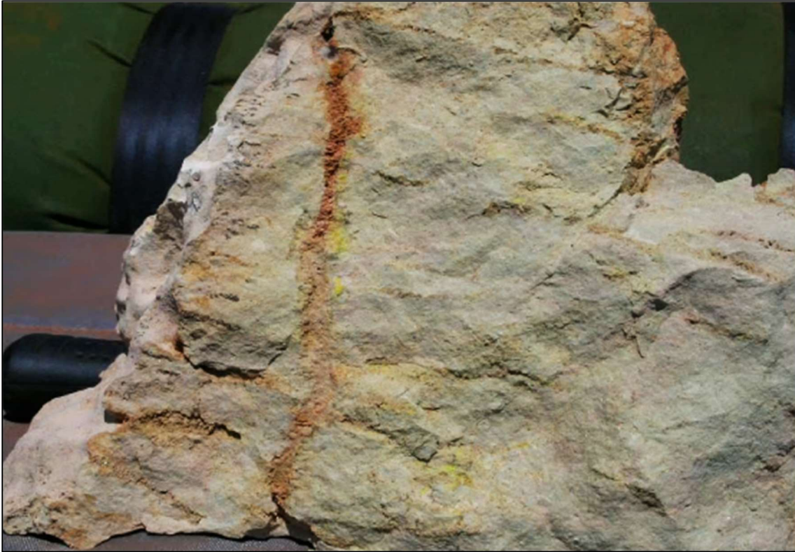
Figure 15: Carnotite (uranium) mineralisation (yellow mineral) in porous sandy limestone from the Ben Hur prospect.
