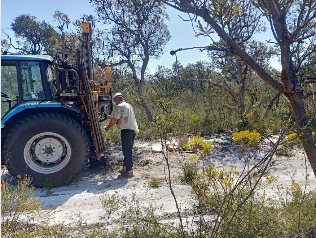
Figure 4: Vacuum drilling at Muchea
