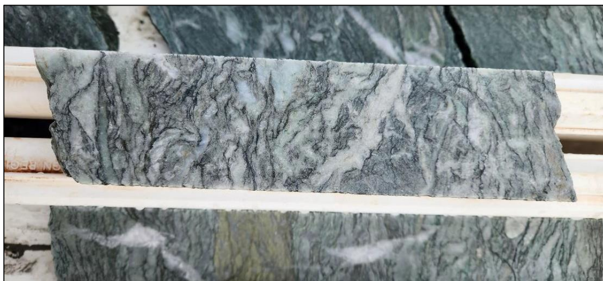
Figure 18. MLJDD018_198.0m Vuggy Silica Alteration
