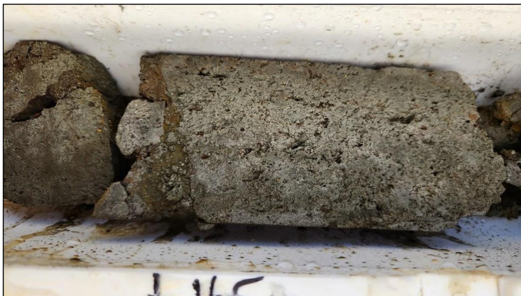
Figure 17. MLJDD018_164.5m_Massive pyrite in Breccia
