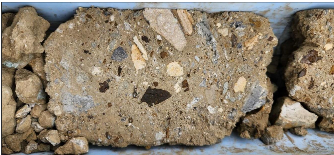
Figure 15. MLJDD020_178.0m_Polymictic Breccia with silica-pyrite clast
