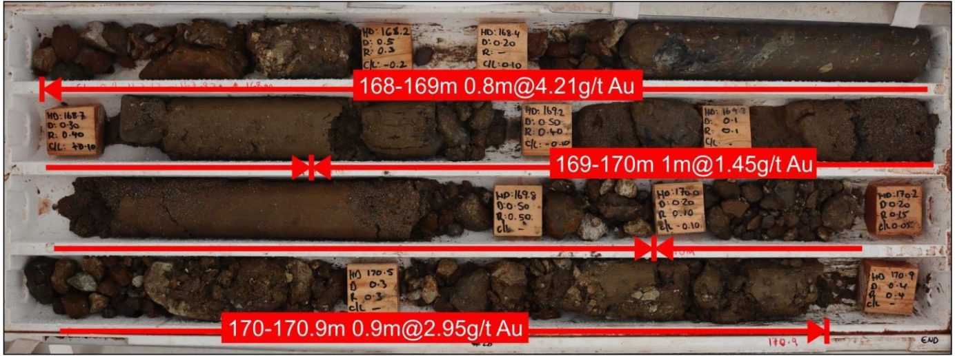
Figure 23. MLJDD015 Breccia alteration
