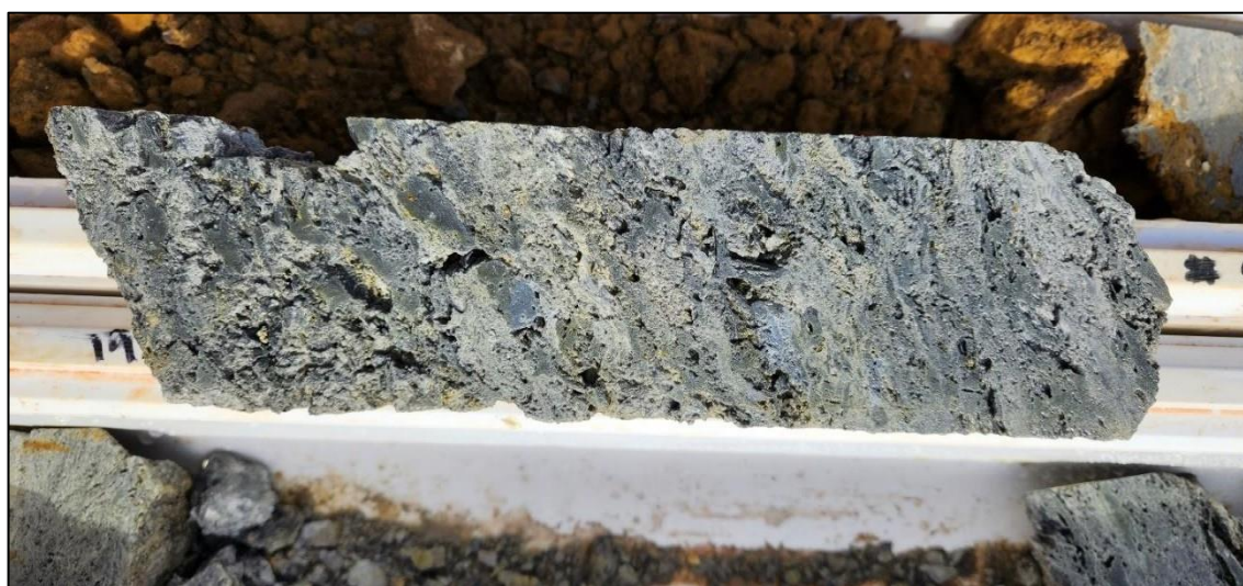
Figure 18. MLJDD018_198.0m Vuggy Silica Alteration
