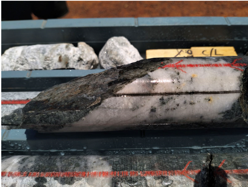
Figure 6, Orientated diamond core with mineralisation in quartz veining
