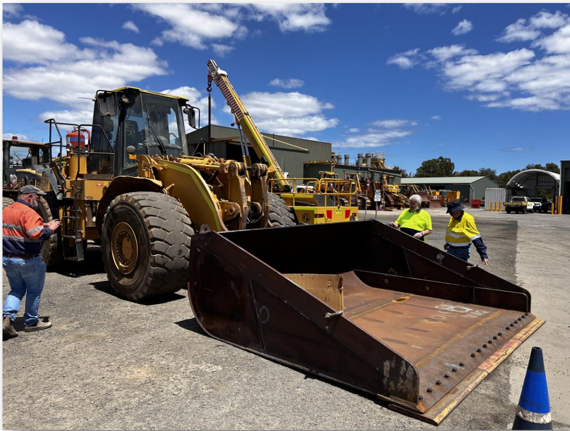
Figure 3: Modified front-end loader bucket for VDT mining method
