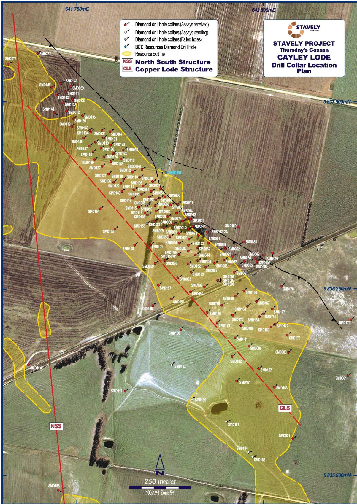
Figure 4. Drill Hole Location Plan on aerial photo.
