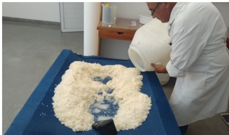
Figure 9: Salt Precipitation Stage, with concentrated brine separate from Salts
