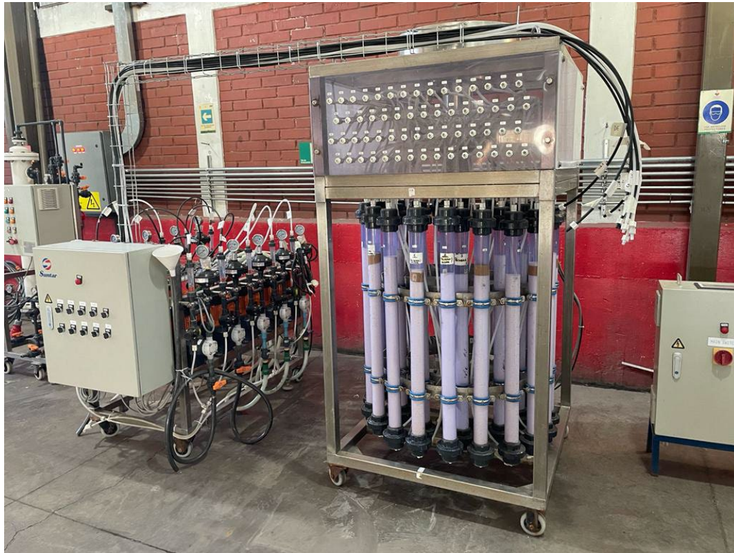
Figure 14: Lanshen Laboratory Scale Continuous Operation Carousel with Lithium Adsorbent
