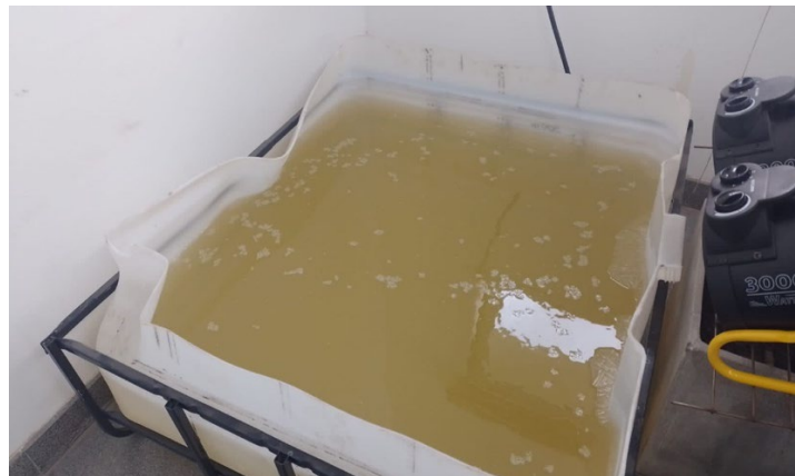
Figure 8: Primary Evaporation Stage of Solaroz Brines
