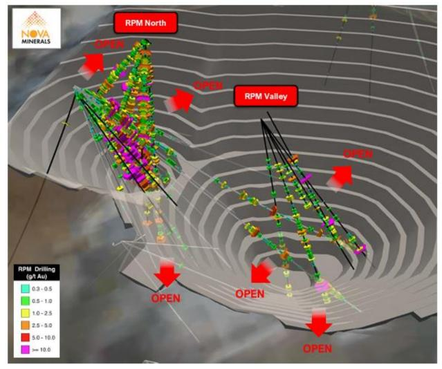
**Figure 4.** 3D Vrify model view looking at RPM North and RPM Valley to the East with the scoping study open pit shell. The arrows show the deposit remains wide open in many directions. New 2023 drill results have black line drill traces
