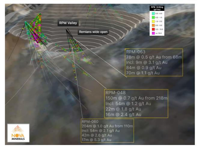
Figure 3. 3D Vrify model looking at RPM Valley with 2023 drill result highlights
