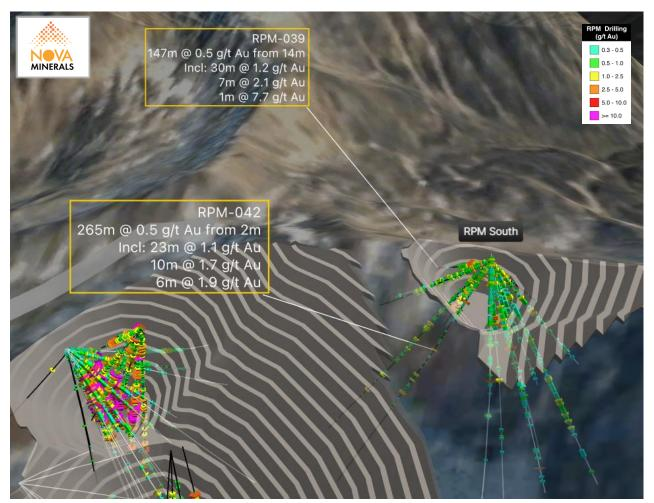
Figure 2. 3D Vrify model looking at RPM South with 2023 drill result highlights
