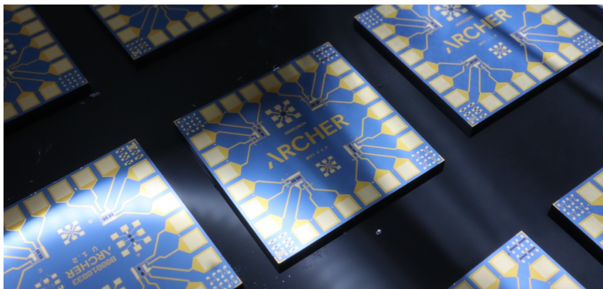
Image 4. Archer's advanced gFET chips diced from the whole four-inch wafer fabricated in a commercial foundry in the Netherlands.
