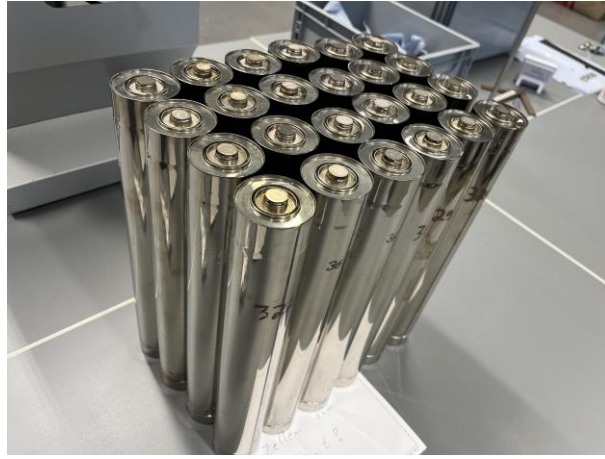
Figure 3 – Some of the completed battery cells waiting performance testing
