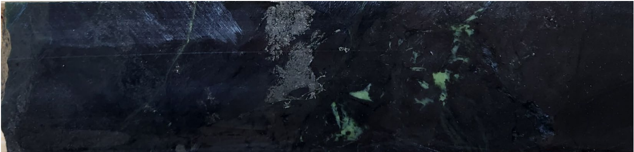
Figure 5: DDED23-143 nickel sulphides (pentlandite-pyrrhotite) in altered peridotite
