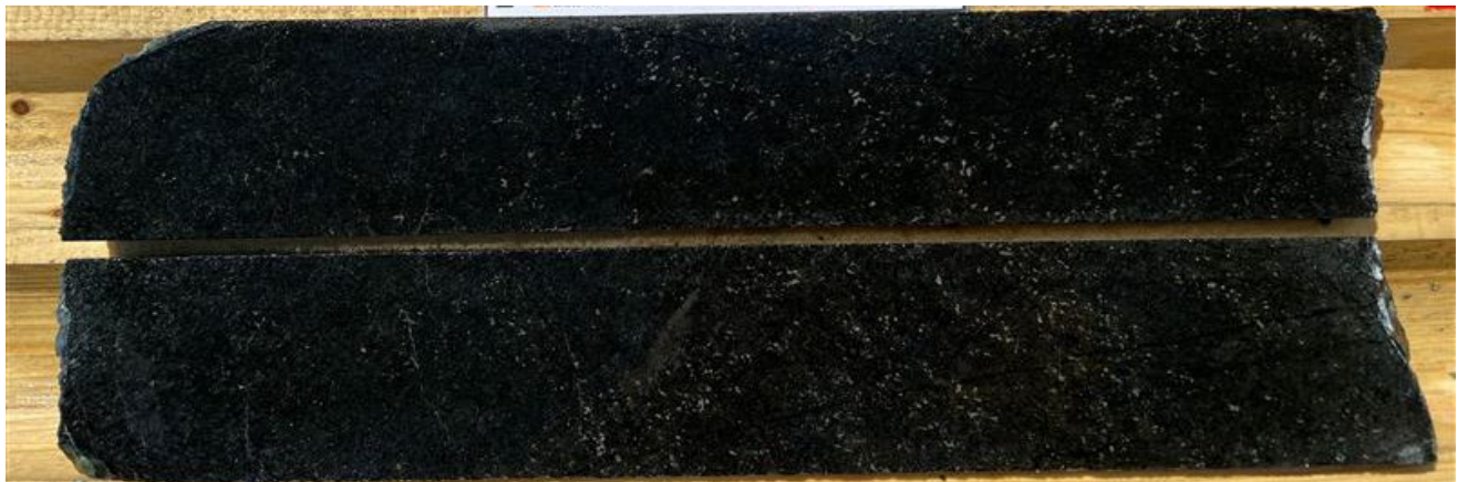
Figure 2: DDED23-131 interstitial to disseminated sulphide mineralisation
