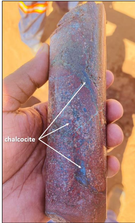
Figure 3: Chalcocite disseminations and veinlets (metallic grey) in weathered biotite schist DBRD149 between 39.55 – 41.47m down hole
