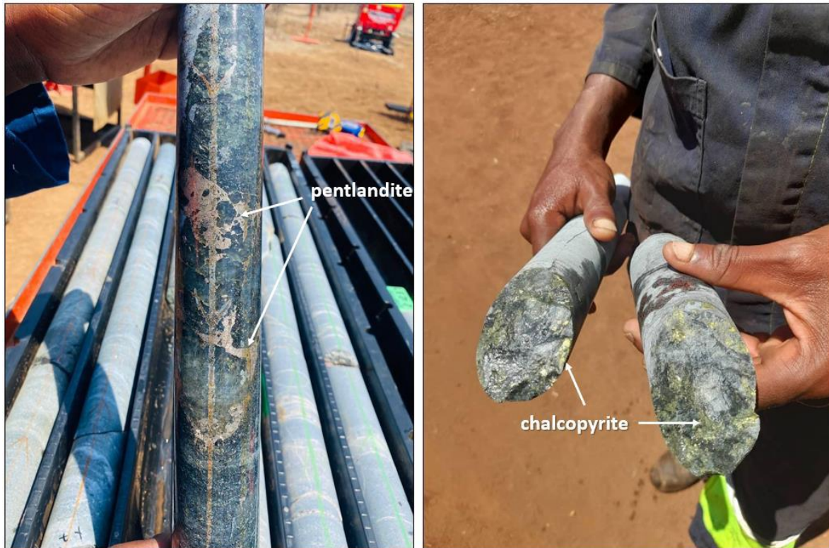
Figure 6: Ni and Cu sulphide examples. Left: Pentlandite semi-massive texture in amphibolite in MARD160 at 208.11 – 208.70m. Right: Chalcopyrite veinlets logged in MADD155 at 187.50m.
