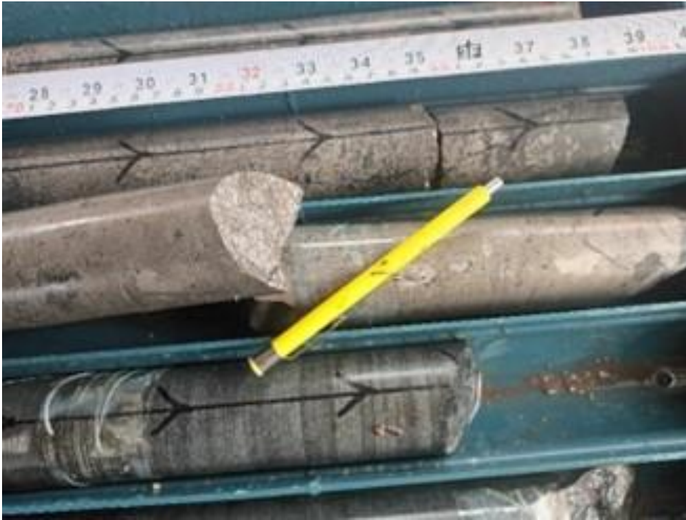
Figure 2: Massive sulphide unit from 423.4m to 423.6m DDLUHC005.
