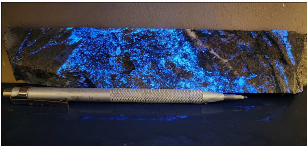
Figure 6: 2019FTD007E, 129.8m - Same segment of drill core under ultraviolet light, highlighting intense scheelite (CaWO 4 ) mineralisation (blue) (Interval 129.5-130.0m Assay: 0.5m @ 6.64g/t Au, 0.38% Co, 1.02% WO 3 , 0.11% Cu ).
