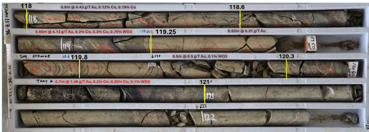
Figure 7: Drill hole 2019FTD004E - Fine grained volcanoclastic sandstone grading into laminated volcanoclastic siltstone with stockwork quartz-carbonate-sulphide veining to 120.3m, then laminated crackle brecciated siltstone with semi-massive pyrite-arsenopyrite-chalcopyrite-galena-pyrrhotite to 121m.
