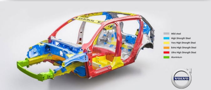
ADVANCED HIGH STRENGTH STEEL UTILISATION IN VOLVO SUV 3
