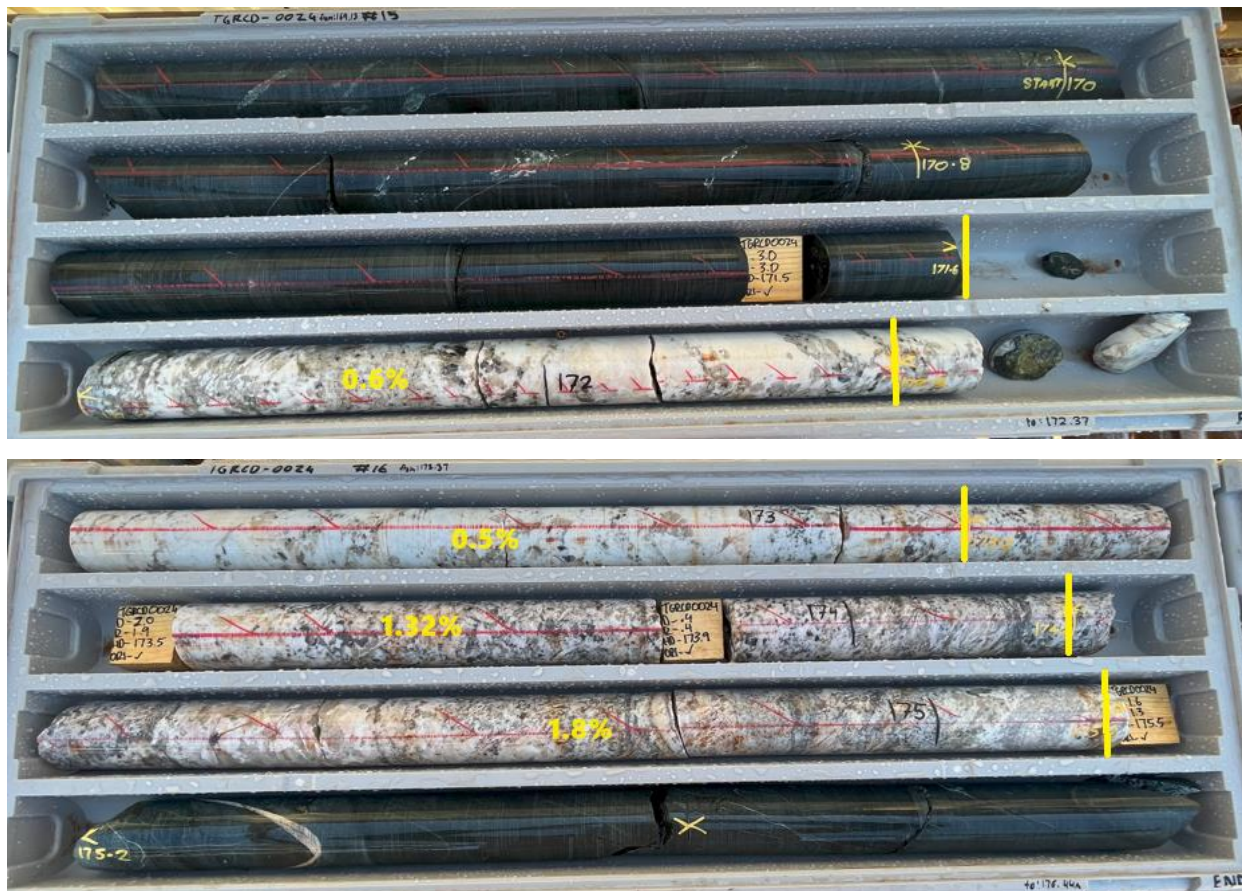
Figure 2: Core from TGRCD0024 pegmatite interval 171.6m to 175.2m pegmatite with Li 2 O% assays
