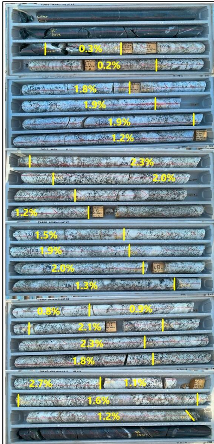
Figure 3: Drill core from TGRCD0024 pegmatite interval 203.7m to 221.5m with Li 2 O% assays – typical of the Burmeister prospect, the entire pegmatite interval is mineralized.
