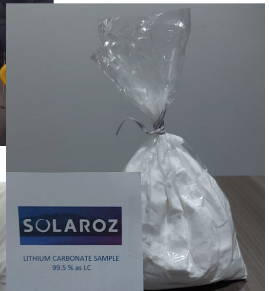
Figure 4: Final Battery Grade 99.5% Lithium Carbonate produced from the Solaroz Brine
