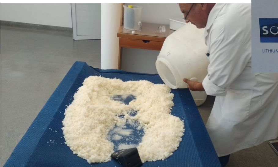
Figure 3: Salt Precipitation Stage, with concentrated brine separated from Salts
