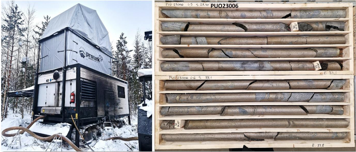
Figure 2: Photograph of the drilling rig on-site at Puolalaki and massive sulphide mineralisation in drillhole PUO23006, (28.4-37.8m).
