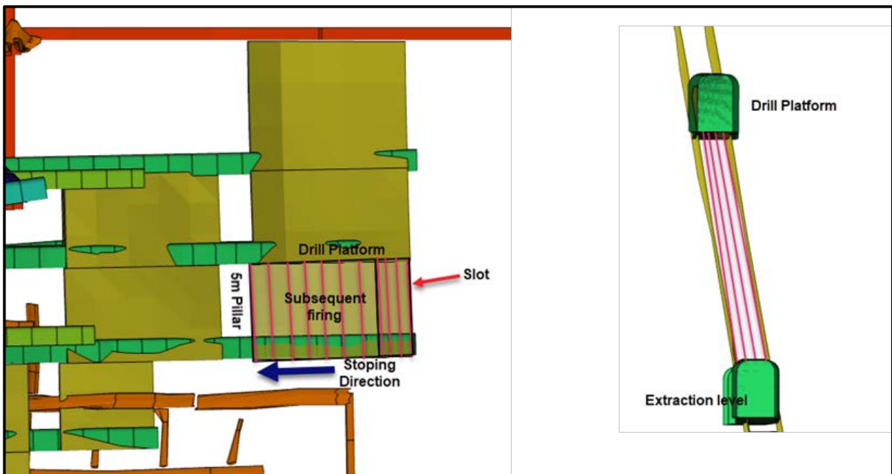
Figure 12 - Proposed Reward Stope Extraction Strategy (Long and Cross section)
