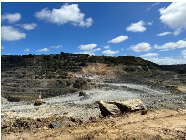
Figure 1 - Preparation of benches on the eastern side of the Dolphin Pit in preparation for mining of high-grade ore
