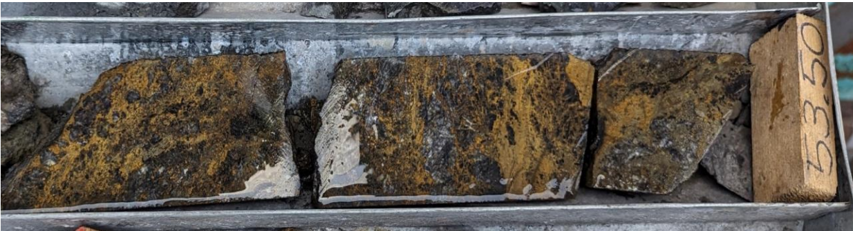
Diagram 8. High-grade copper mineralization at Sabana Blanca semi-massive to massive chalcopyrite mineralization in a heavily veined zone
