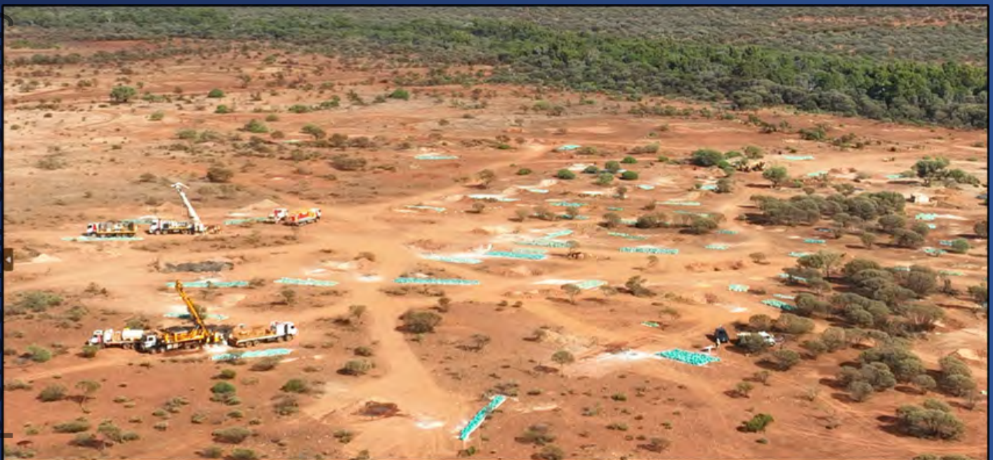
Figure 2. Two Drilling Rigs (1x RC, 1x Diamond) Drilling SEB zone at Crown Prince (September 2023)
