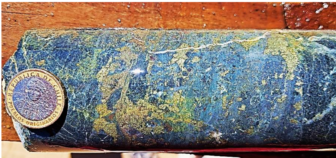
Figure 1: Shallow visible copper mineralisation intersected over 40m in drillhole CMEQD002.
