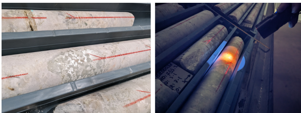
Figure 2:(Left) Coarse spodumene in dry core; (Right) Spodumene fluorescing orange under a UV lamp as part of the standard logging process.
