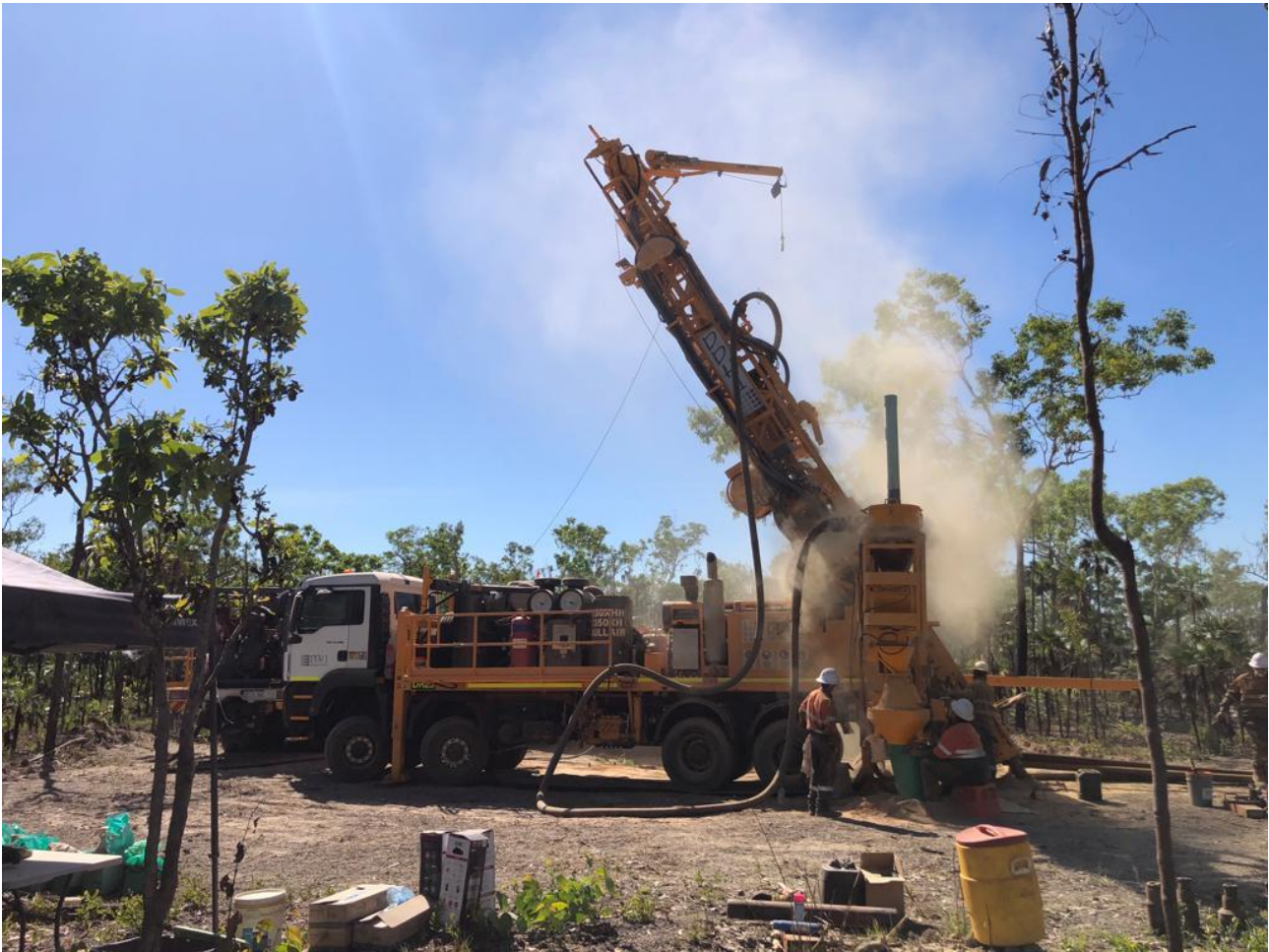
Figure 3: Dual RC/DD rig in operation at Perseverance Prospect, Kings Landing Area
