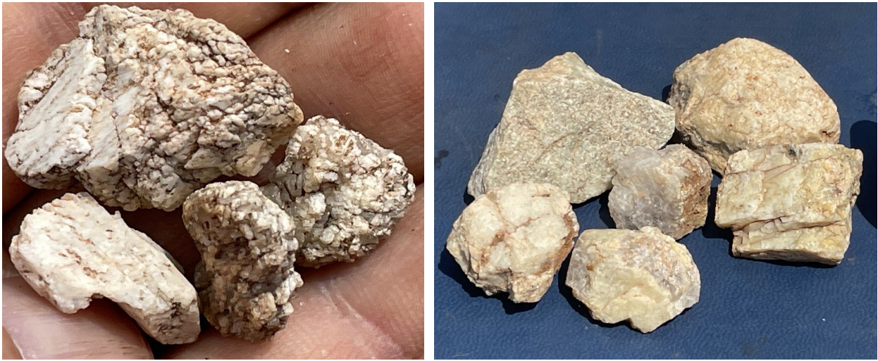
Figure 4 - Weathered pegmatite drill chips from historic drill hole JBR110 (left), and weakly sericitic pegmatite drill chips from historic drill hole JBR117 (right)
