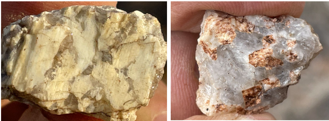
Figure 3 - Example of weakly weathered pegmatite drill chips observed in historic drill hole JBR296 (left), and strongly weathered pegmatite from historic drill hole JBR140 (right)
