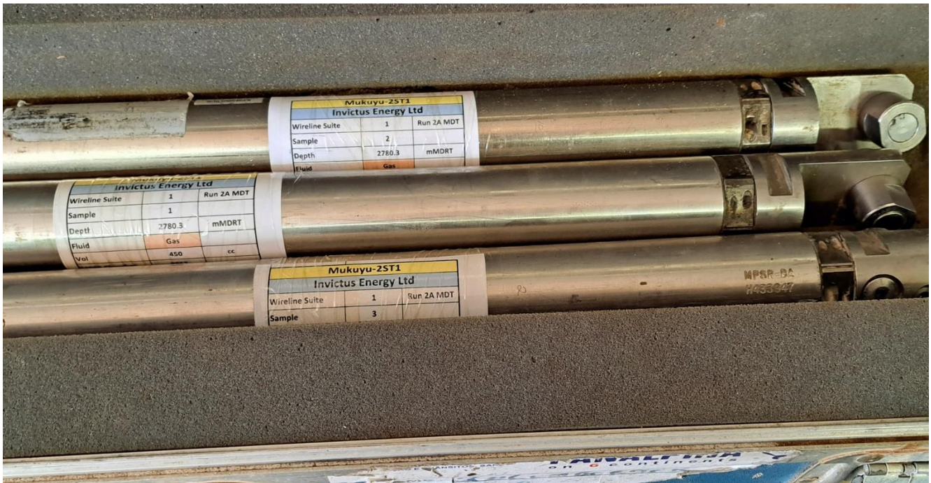
Figure 1 - Pressurised sample chambers containing gas recovered to surface from Mukuyu-2 sidetrack in preparation for shipping for laboratory analysis
